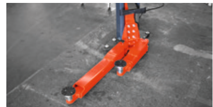
Parallel position of the swivel arms possible, for easier and faster positioning of the vehicles
