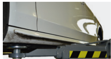
Low arm construction <100mm
