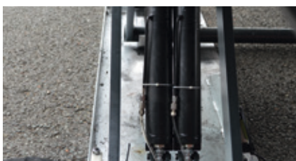
Double hydraulic system, therefore no compressed air required
