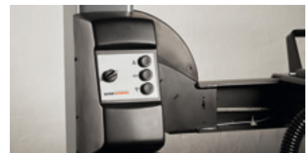
Pump and control unit on front left post
