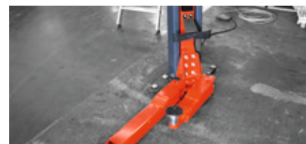
Arms can be opened more than 180° for better drive-in situation for lifts installed in 90° angle to the drive lane
