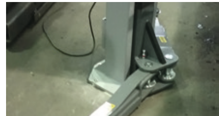
Swivel arm positioning > 180° for better drive-in situation
